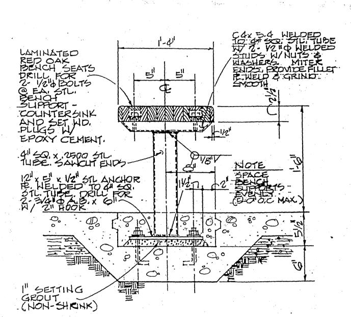
TYPICAL WD. BENCH DETAIL @ NEW FLOOR SLAB ON GRADE
